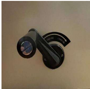
Fig. D.3 Unloading and Loading position
