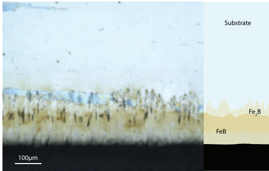
Figure 5.11: On the left an optical image of the microstructure of BB, and on the right a schematic describing the various layers.
