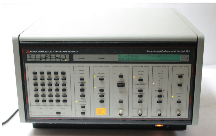
Figure 3.7: Princeton Applied Research model 273A potentiostat/galvanostat front panel [66].
