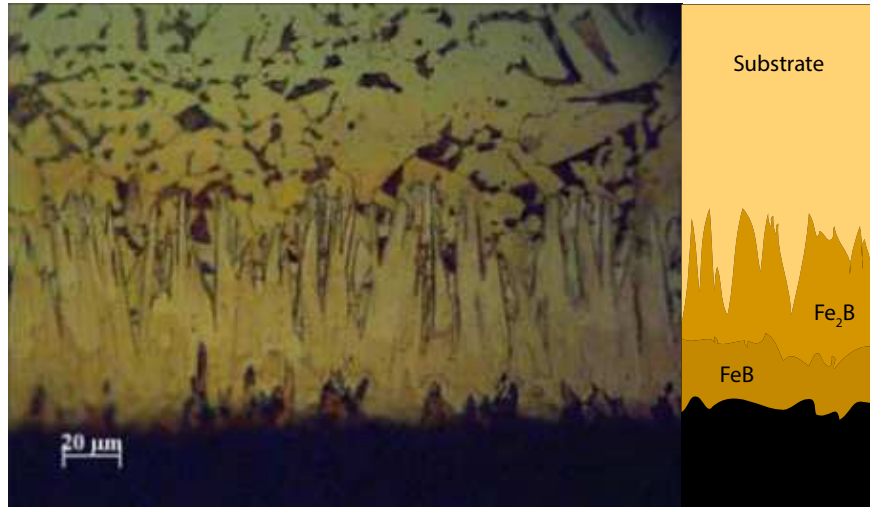
Figure 2.3: On the left an optical image of the microstructure of boronized low-carbon steel (AISI 1018), and on the right a schematic describing the various layers [6].
