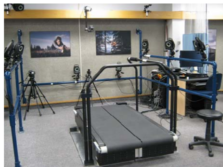
Figure 4 Treadmill for marker-less motion capture system testing.
