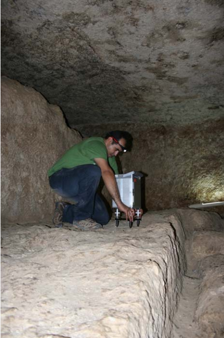
Dr. Elhabiby at the Subterranean room 120ms under the Great Pyramid- Gravimetry Measurements
