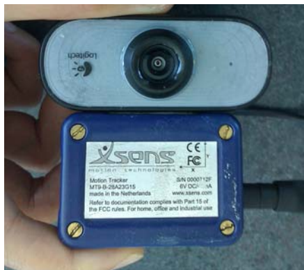
Figure 1. A consumer-grade MEMS IMU by Xsens and a low-cost webcam by Logitech
