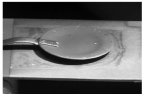
Fig. 29. Suspended structure: Cantilevered capacitor plate (12 mm diameter).
