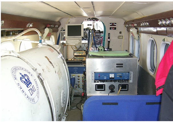
Fig. 4. Cabin set-up: extended-range ferry tank (left), rack and aluminum cage with gravimeter.
