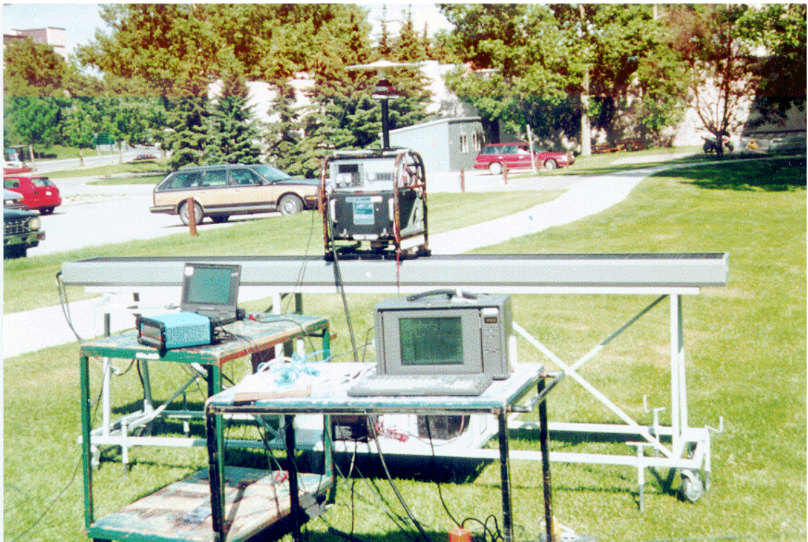
Fig. (8.1) : INS/GPS on Anorad Platform (Anorad Test Setup)
