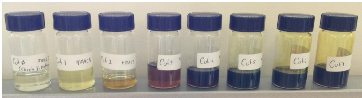
Figure 4.7. Photograph of the seven different cuts of WC-B-B1 maltenes from Fractionation 4 (DVFA-II).
