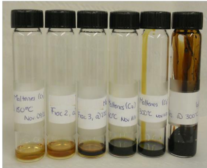
Figure 4.2. Photograph of five different cuts and residue of WC-B-B1 maltenes from Fractionation 1 (DVFA-I) proof-of-concept test.
