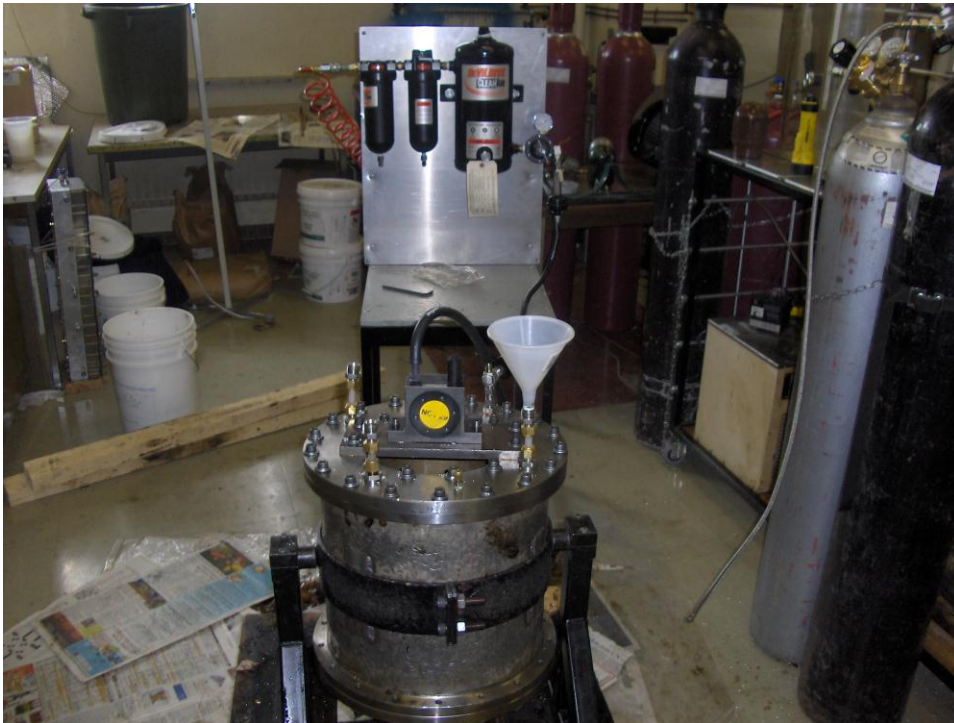
Figure 6-4: Packing the Vapex physical model with 12-16 U.S. mesh glass bead.
