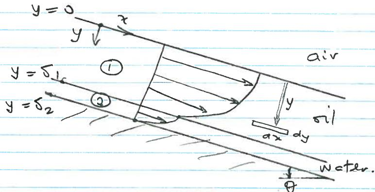
Locate origin at air-oil interface as shown in diagram.
