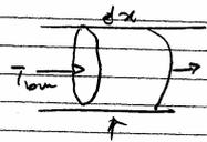
$$\text{or} \quad \frac{dT_{bm}}{dx} = \frac{2 q_w}{RV \rho c_p} = \text{const.} \quad (2)$$
