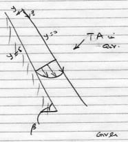
Set up the problem by toknow? a deferential element in the film - person a force belance to state the velocity distribution and a mass belowed on the acid (TA).
