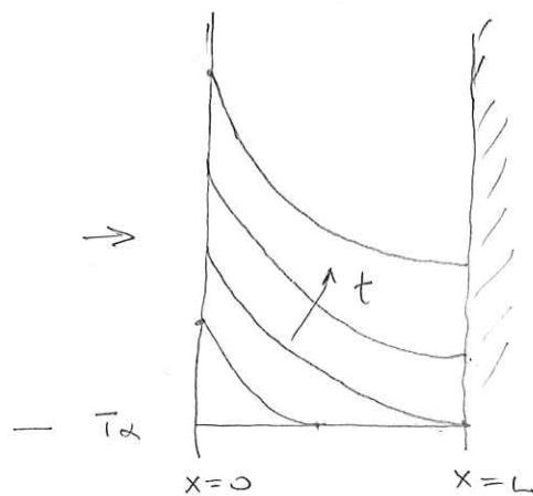
In the tile, the rates of absorption  $q_a$  and convection  $q_c$  will change with time.
