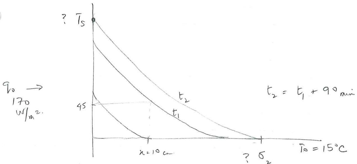
Required to find  $\delta_2$ ,  $\int_{T_0}^{T_2} \rho C_p (T - T_0) dx$  or  $q_0 \cdot t_2$  and  $T_s$ .
