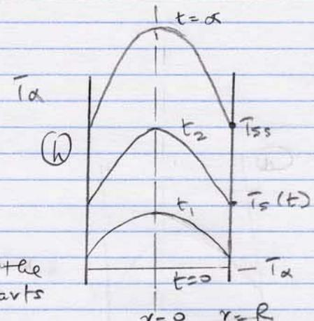
The time-dependent temp. pattern in the rod is sketched to the right. The rod starts at a uniform temperature  $T_a$ . As heat is generated, some is stored in the rod and the rest is transferred into the pressurized water at  $T_w$ .
