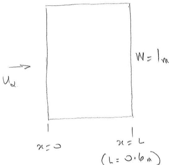
The problem has two parts. Pressure due to the velocity head pushes on the front surface, and shear stress acts on the 4 lateral walls. The back wall has no contribution.
