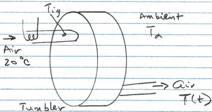
The hot air leaving the tumbler is assumed to be at the same temperature as the clothes and the tumbler.
