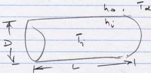
Assume the fuselage or plane body is a cylinder closed-ended by flat plates.
