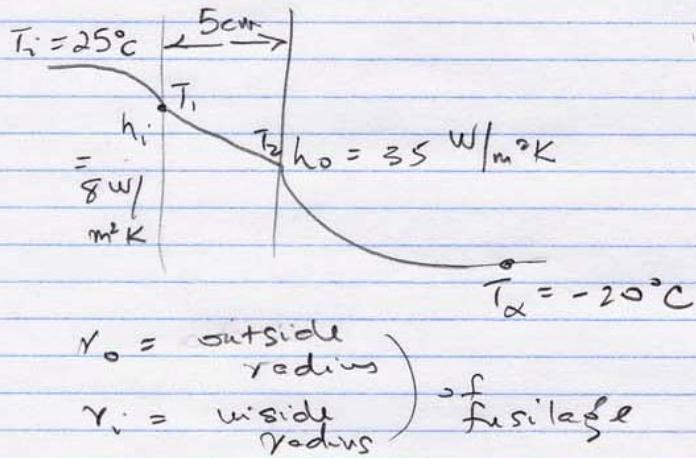
From the curved wall, the heat transfer rate is given by (see sketch)
