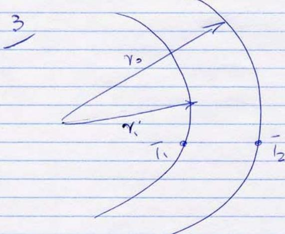
$$Q = 4\pi k \frac{(T_1 - T_2)}{\frac{1}{r_i} - \frac{1}{r_o}}$$
