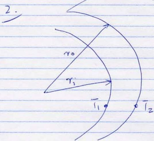
$$Q = \frac{2\pi k L (T_1 - T_2)}{\ln(r_o/r_i)}$$
