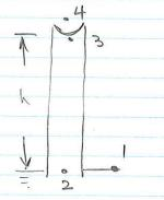
water is pulled up by surface tension forces and resisted by gravity. Choose points 1-4, as per sketch.
