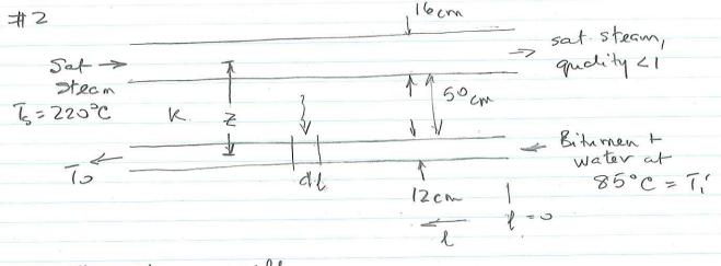
The steam well will trensfer heat to the producing well. Harough the soil.
