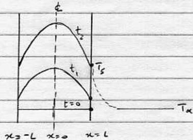
Because  $h$  is finite, and conditions on both sides of the plate are identical, the temperature profiles are approximately as illustrated with the surface temperature,  $T_s$ , time-dependent. In the body,  $T = T(x, t)$ .
