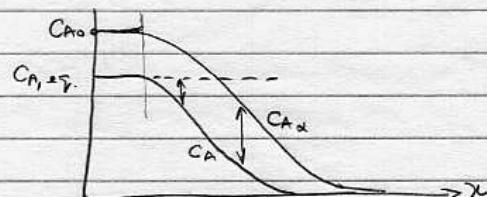
Mass Transfer into each particle (local condition).
