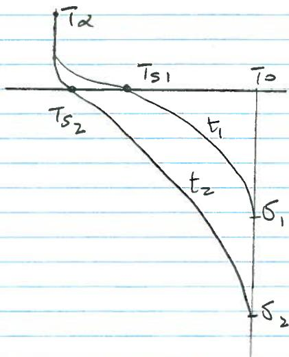
This is a problem of heat transfer into a semi-infinite domain, with a convective boundary condition.
