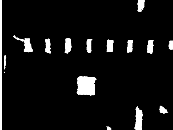
Figure 5.11: The binary image after depth-based segmentation (Kinect)
