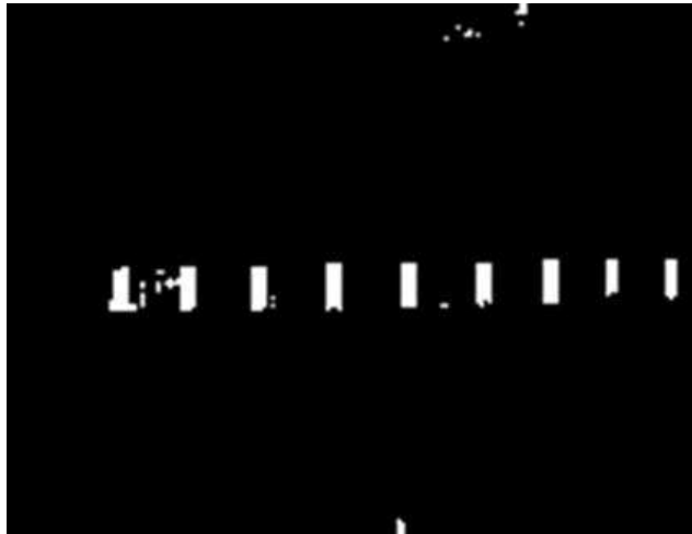
Figure 5.5: The binary image based on Otsu threshold method (SR4000)
