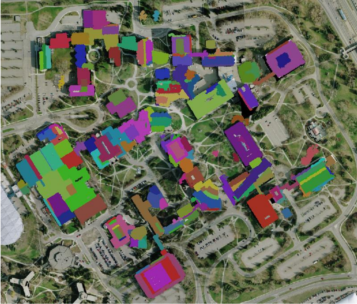
Figure 6.4: Generated building hypotheses from LiDAR data overlaid on top of an orthophoto
