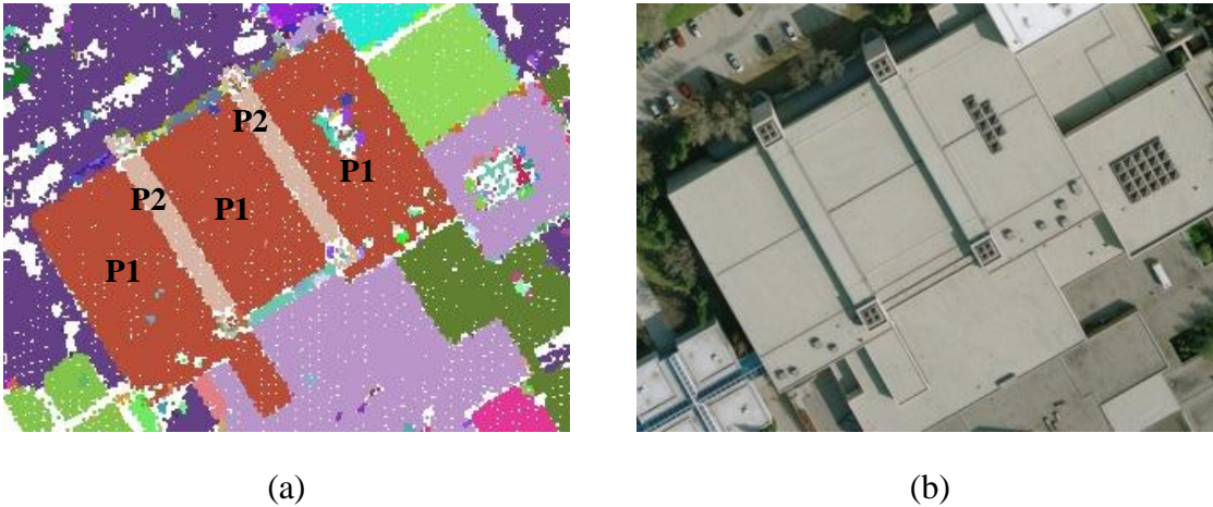
Figure 3.6: The ambiguity problem of parameter-domain segmentation: planar region segmentation (a) and aerial image over the same planar surface (b)
