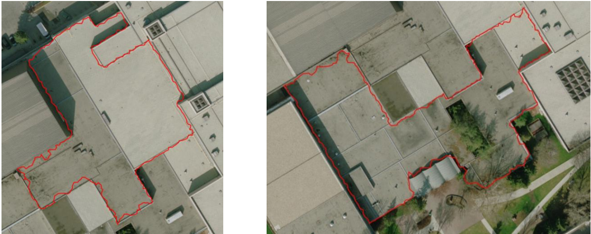
Figure 3.13: Example of projected LiDAR boundaries onto an image
