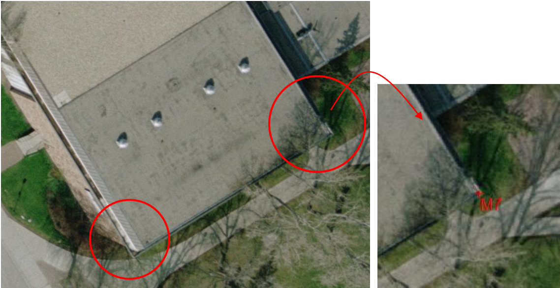
Figure 6.23: Problems with manually-identified corner points
