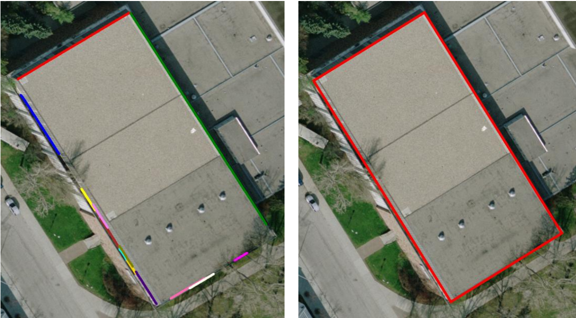
Figure 6.23: Problems with manually-identified corner points
